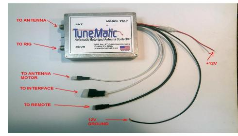
1) 12v power leads: These leads can be paralleled with radio power if desired, as they draw no current until TuneMatic is powered up by Radio Control cable. <u>NEGATIVE GROUND</u> SYSTEM ONLY!
